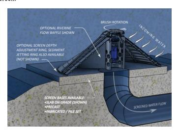
The inlet structure for the cone screen will be set at a lower elevation than the bottom of the low flow channel in order to maintain sufficient depth of water for irrigation diversion. Because this area will likely collect some sediment, a sediment sluicing system could be installed to manage sediment. As sediment collects near the bottom of the screen, a valve or gate could be temporarily opened to sluice the sediment out and discharge it downstream.
