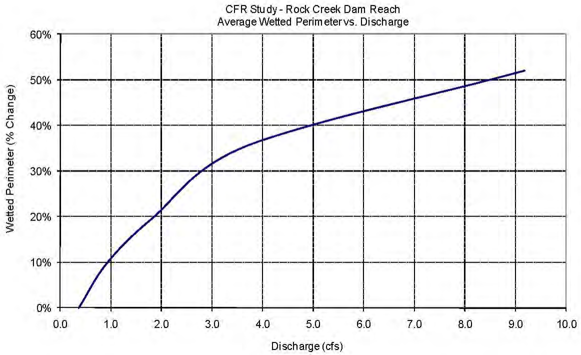
Figure 3-57. Percent change in wetted perimeter as a function of discharge in Rock Creek below Rock Creek reservoir dam, averaged across three channel flow response transects. (Source: Technical Memorandum 3-2, Instream Flow ; NID and PG&E 2010)
