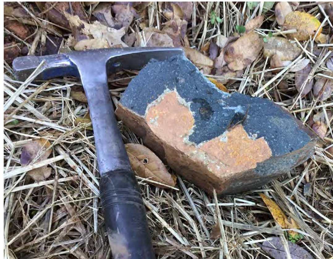
C) Rock sample from Unit LCC-3b of a fine-grained basalt with 1-2 mm long plagioclase and pyroxene phenocrysts. Rock hammer for scale.
