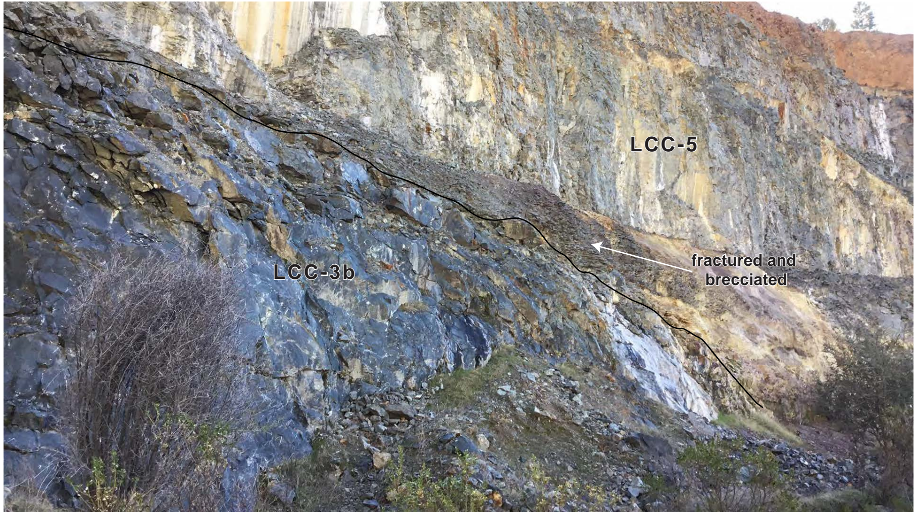
View to the east of the bedding contact between Units LCC-5 (top) and LCC-3b (base) dipping southerly within the eastern part of Teichert Quarry (see Figure 4 for location).
