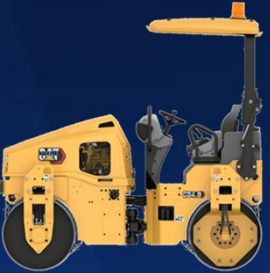
Utility Compaction Roller (asphalt and off-road)
