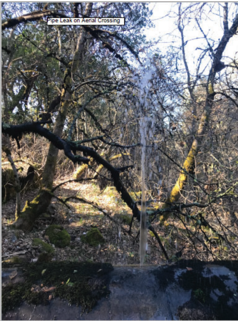
Aerial Pipe Crossing - Severe corrosion and failed pipe wrap/covering
